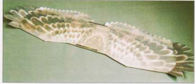
0.02 Insert the 600mm long carbon flat bar into the spare slot on the back of the aerfoil, then paste the other 3pcs 150mm long carbon flat bar with UV glue onto front and back of the main wing. Here the aerfoil part is finished.
